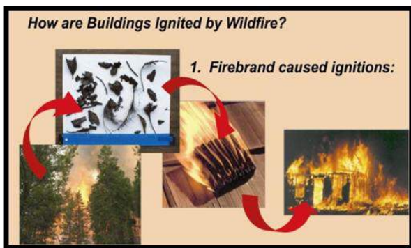
Figure 14. Firebrand caused ignitions: burning embers are carried ahead of the fire front and alight on vulnerable building surfaces.
